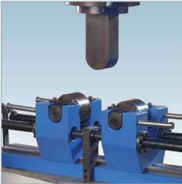
Common Bend Re-Bend & 180° Bend Test Attachment with various diameter mandrels
