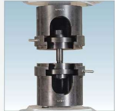
Special Attachment For Short Specimens/ Nut-Bolts
