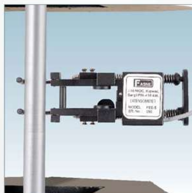
Electronic Extensometer (Model: FEE-5)
